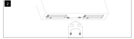
Fix the fixture to the unit using 2 fixing screws
