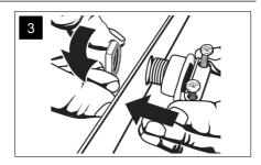
Insert romex connector into the housing open hole on the adapter plate. Secure it with the nut.
