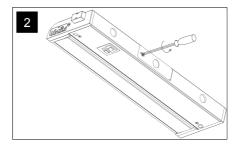
Disengage adapter plate by loosening screw.
