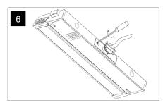
Feed wires back into fixture, reattach adapter plate tighten screw, and attach the fixture to the base of the cabinet, with screws
